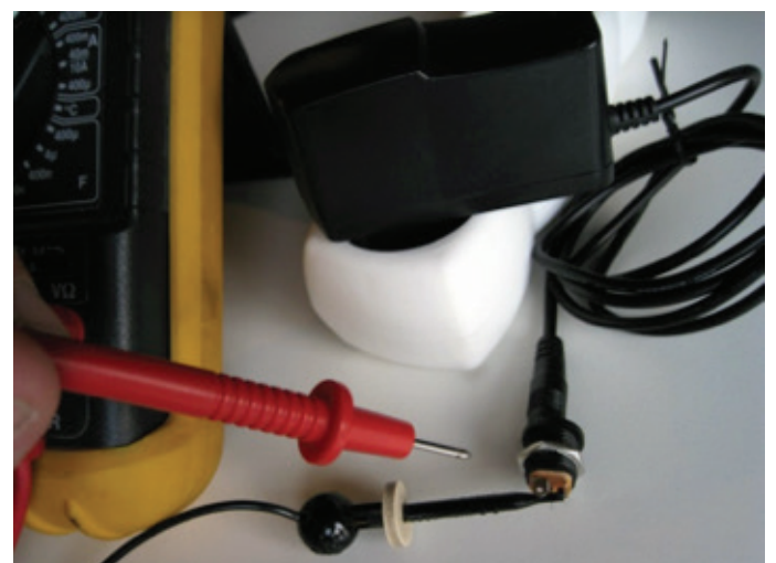
Measure the polarity of the supply voltage before connecting the supply wires!
