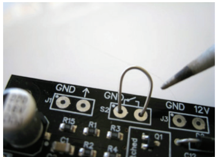
If you don't need the optional footswitch, just add a jumper to enable the tremolo.
